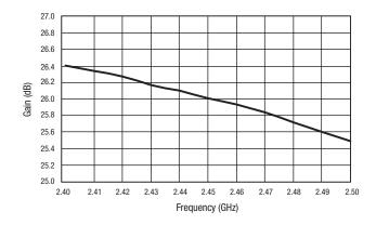
**Figure 4. Typical Gain vs Frequency Response**
