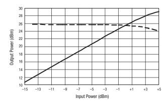
Figure 3. Typical Pout and Gain vs PIN @ 2.442 GHz
