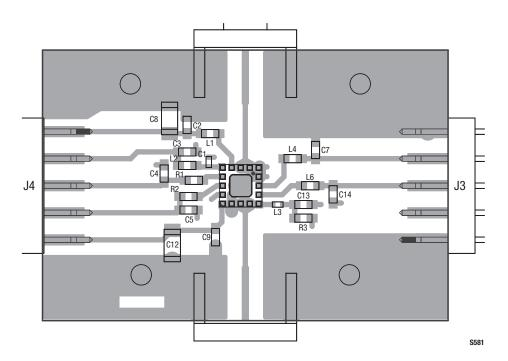
**Figure 11. Evaluation Board Assembly Drawing**
