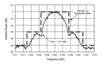
Figure 7. Output Spectrum Response for 802.11b CCK-Coded (11 Mbps Input Signal)
