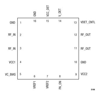
Figure 1. SKY65131 Pinout – 16-Pin MCM (Top View)
