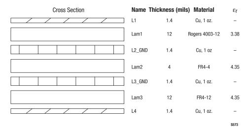
**Figure 13. Layer Detail Physical Characteristics**
