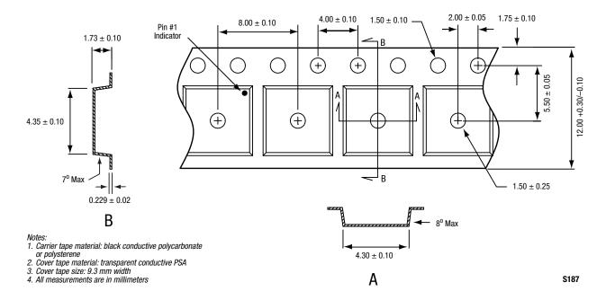
Figure 15. SKY65131 16-Pin MCM Tape and Reel Dimensions
