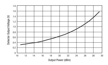
Figure 8. Detector Output Voltage vs RF Output Power
